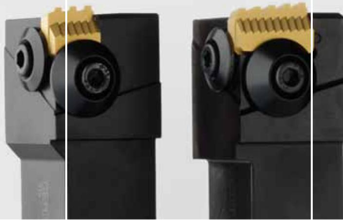
The two-pin system ensures extremely precise insert positioning from insert to insert as well as plays a key role in the holder's increased rigidity. With more rigidity and support, the holder helps reduce the amount of required threading passes for generating a full thread profile.
